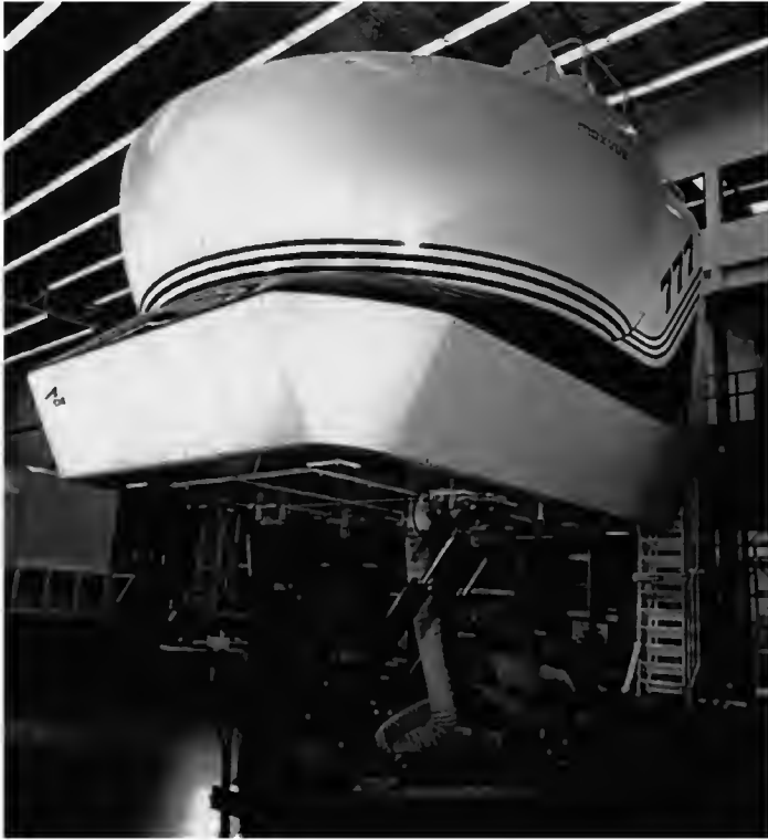
FIGURE 1.5. A six-degree-of-freedom flight simulator (courtesy of CAE Electronics Ltd.)
